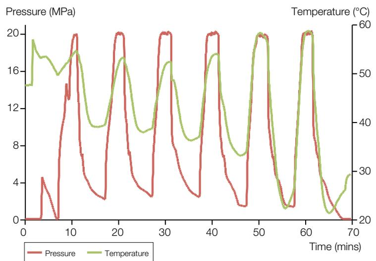
Figure 2: Supercritical CO<sub>2</sub> dewatering of radiata pine showing the pressure cycling. The internal temperature of the sample increasingly rises and falls with each cycle as sap is removed and more CO<sub>2</sub> can enter the wood. This results in an increased temperature via heat of compression of extra CO<sub>2</sub> and then decreased temperature due to increased decompressive cooling of the extra CO<sub>2</sub> as it changes into a gas. The vessel jacket was maintained at 50°C
