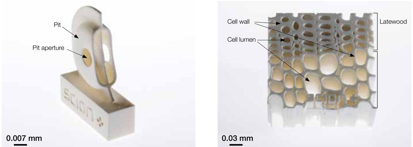
Figure 1: 3D printed objects showing anatomical structure of radiata pine. Left: Pit structure. Right: Tracheid structure. Scale bars give indicative size. Any size for 3D printed models can be selected (e.g. 50 mm)
