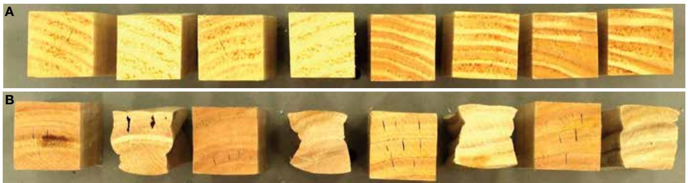
Figure 5: Four sets of duplicates showing collapse (end grain view) for: a) radiata pine; and b) *Eucalyptus regnans*. Repeating from left to right: 'dewatered and oven dried' to 'oven dried only'. Sample size was 37 x 37 x 200 mm (radial x tangential x longitudinal)
