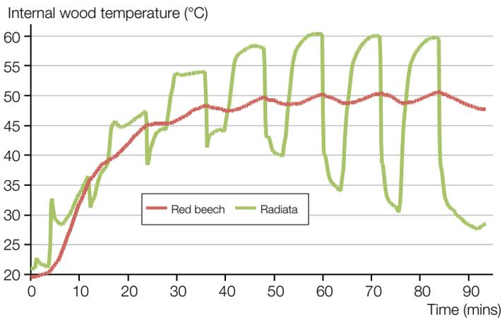
Figure 4: Supercritical CO<sub>2</sub> dewatering of radiata pine and red beech showing the internal temperature of the samples. The red beech gravitates to the vessel jacket temperature of 50°C, indicating there is no dewatering occurring
