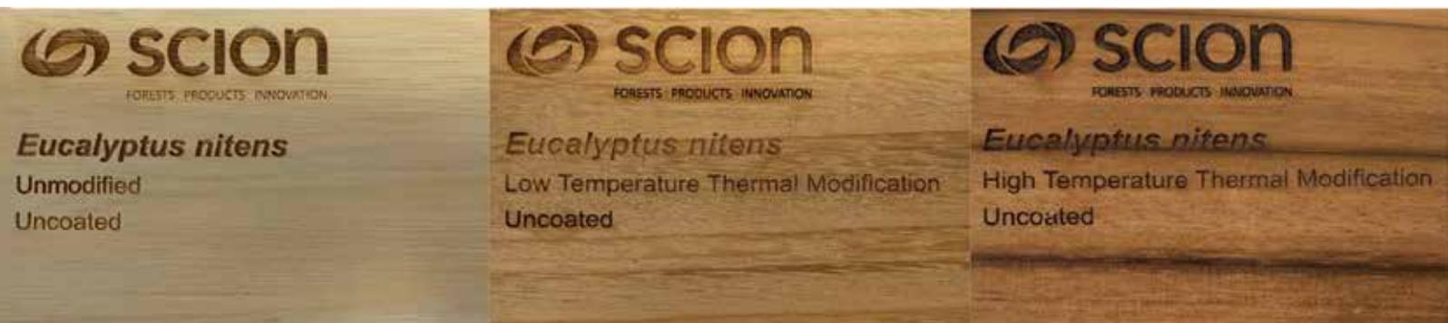
Figure 1: From left to right, the colour of untreated and heat-treated *Eucalyptus nitens* at low and high temperatures. Source: Scion
