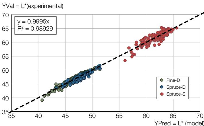
Figure 3: PLC model for colour of thermally modified spruce and pine
